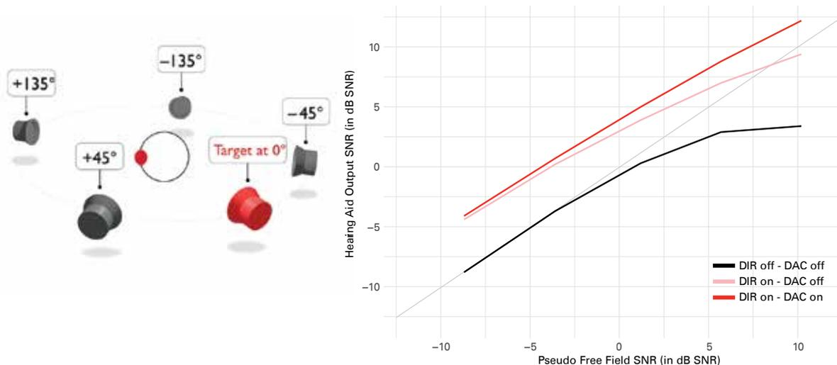
On the left, spatial distribution for speech, the target signal, in red and noise sources in gray for output SNR measures. On the right, a graph of the output SNR with compression plus three different feature configurations: black, compression only; pink, directionality and compression; and red, directionality, DAC™, and compression activated. The straight light gray curve shows values where the input SNR on the horizontal axis equals the output SNR on the vertical axis.
