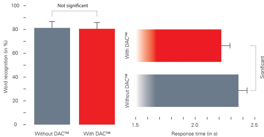
Results from word recognition tests with DAC™ deactivated in gray and DAC™ activated in red. Performance is measured with word recognition percentage on the left side and with response time in seconds on the right side. Average performance and one standard error are shown on the graphs.
