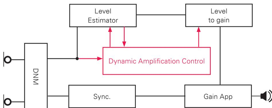
Block diagram of the implementation of the Dynamic Amplification Control™ algorithm between the Dynamic Noise Management™ block and the compression unit.
